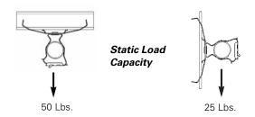
Note: An independent means of support is required by NEC Article 300.11. Refer to pages 221-222 for additional support methods.
